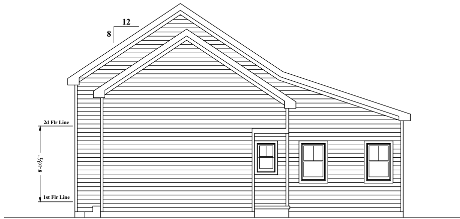
Right Side Elevation 1/4" = 1'-0"
